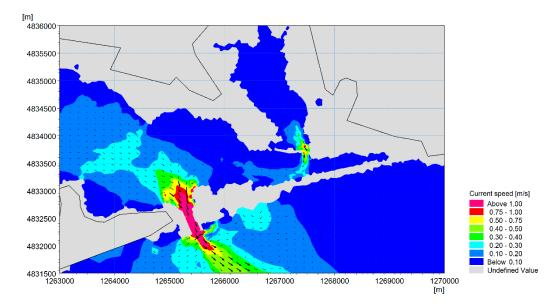
Figure 3-11 Current speed three hours after commencement of simulation for areas with the main *Ruppia* beds as elevated water levels drain out of lagoon for Hansen's Bay with no sill.
