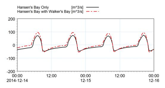
Figure 3-18 Comparison of flow through Hansen's Bay spit breach for only Hansen's Bay breach and combination of Hansen's Bay and Walker's Bay breaches for approximately neap tide. A positive flow indicates flow into the lagoon while a negative flow indicates flow out of the lagoon.
