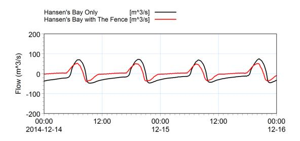
Figure 3-19 Comparison of flow through Hansen's Bay spit breach for only Hansen's Bay breach and combination of Hansen's Bay and The Fence breaches for approximately neap tide. A positive flow indicates flow into the lagoon while a negative flow indicates flow out of the lagoon.
