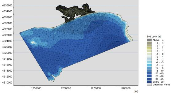
Figure 3-1 Hydrodynamic model extent – bathymetry (top) and mesh (below).
