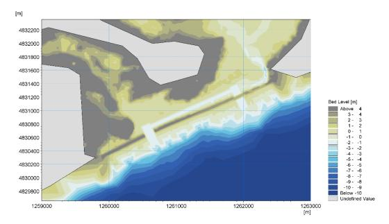
Figure 3-12 Bathymetry for Walker's Bay western opening.
