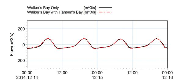
Figure 3-17 Comparison of flow through Walker's Bay spit breach for only Walker's Bay breach and combination of Hansen's Bay and Walker's Bay breaches for approximately neap tide. A positive flow indicates flow into the lagoon while a negative flow indicates flow out of the lagoon.
