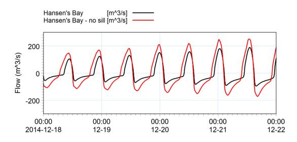
Figure 3-9 Comparison of flow through Hansen's Bay opening with and without the sill for approximately mean tide. A positive flow indicates flow into the lagoon while a negative flow indicates flow out of the lagoon.
