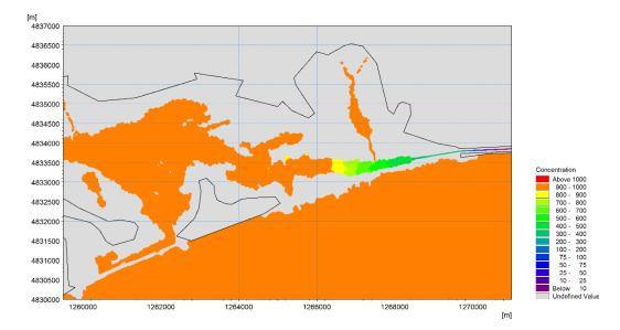
Figure 3-28 Final concentration of a conservative tracer with an initial concentration of 1000 in lagoon and river boundary condition of zero concentration, to predict the tidal flushing that may occur after a neap spring tide cycle.
