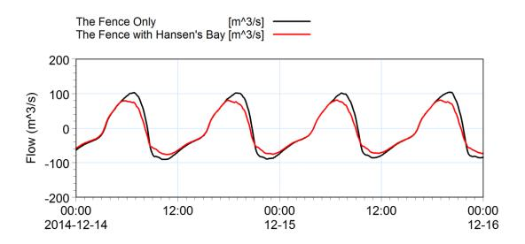
Figure 3-20 Comparison of flow through The Fence spit breach for only The Fence breach and combination of Hansen's Bay and The Fence breaches for approximately neap tide. A positive flow indicates flow into the lagoon while a negative flow indicates flow out of the lagoon.
