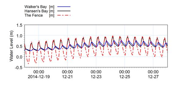
Figure 3-8 Comparison of water levels in the lagoon adjacent with Hansen's Bay for different spit openings.
