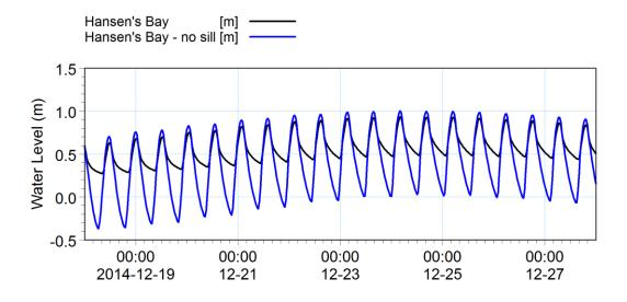
Figure 3-10 Comparison of water level in the lagoon adjacent with Hansen's Bay with and without the Hansen's Bay sill.
