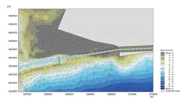
Figure 3-27 Model bathymetry and mesh where the canal and lagoon connect.
