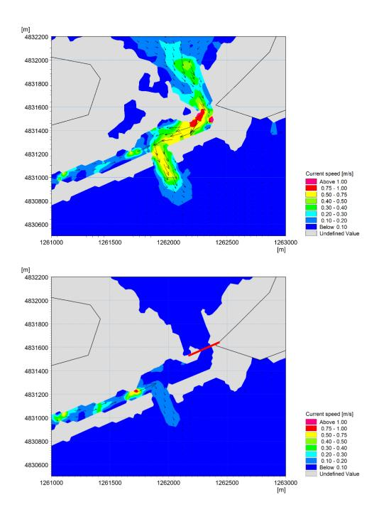
Figure 3-24 Comparison of current speeds for peak ebb tide for a mean tide for Walkers Bay spit opening without (top) and with the internal dike (bottom), indicated by red line.
