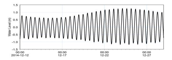
Figure 3-3 Open ocean boundary condition for neap spring tidal cycle.
