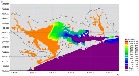
Figure 3-5 Final concentration of a conservative tracer with an initial concentration of 1000 in lagoon and zero in open ocean, to predict the tidal flushing that may occur after a neap spring tide cycle for different spit openings – Walker's Bay (top), Hansen's Bay (middle) and The Fence (bottom).
