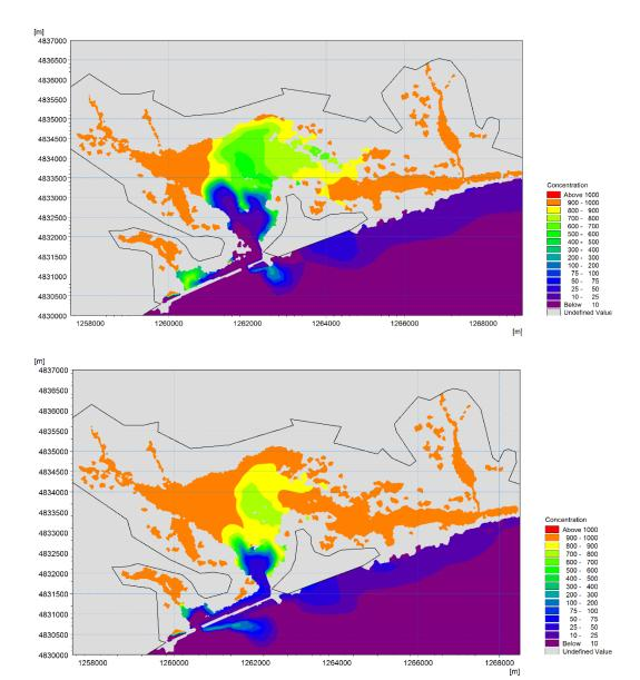
Figure 3-15 Final concentration of a conservative tracer with an initial concentration of 1000 in lagoon and zero in open ocean, to predict the tidal flushing that may occur after a neap spring tide cycle for Walker's Bay opening located to east (top) or to west (bottom).
