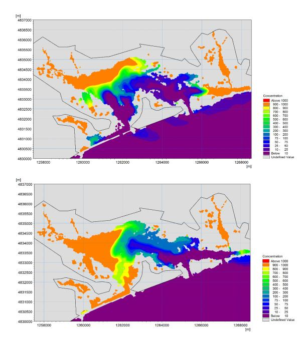
Figure 3-16 Final concentration of a conservative tracer with an initial concentration of 1000 in lagoon and zero in open ocean, to predict the tidal flushing that may occur after a neap spring tide cycle for different combined spit openings – Walker's Bay and Hansen's Bay (top) and Hansen's Bay and The Fence (bottom).
