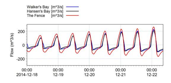
Figure 3-6 Comparison of flow through different spit openings for approximately mean tide. A positive flow indicates flow into the lagoon while a negative flow indicates flow out of the lagoon.
