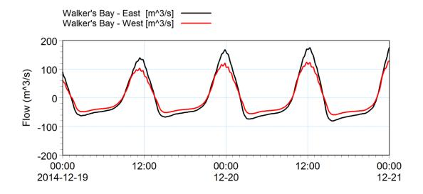
Figure 3-14 Comparison of flow through Walker's Bay opening located to east (current location) or to west for approximately mean tide. A positive flow indicates flow into the lagoon while a negative flow indicates flow out of the lagoon.
