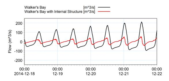
Figure 3-25 Comparison of flow through the Walkers Bay spit opening with and without the internal dike. A positive flow indicates flow into the lagoon while a negative flow indicates flow out of the lagoon.
