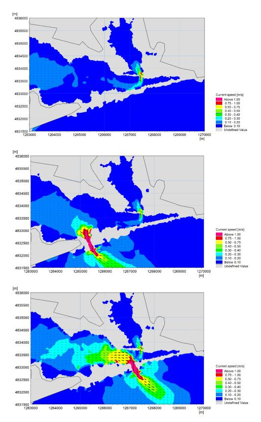
Figure 3-7 Current speed three hours after commencement of simulation for areas with the main *Ruppia* beds as elevated water levels drain out of lagoon with different spit openings – Walkers Bay (top), Hansen's Bay (middle) and The Fence (bottom).
