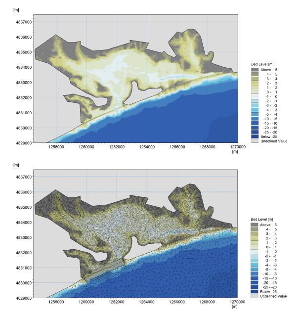
Figure 3-2 Hydrodynamic model lagoon bathymetry (top) and mesh (below).
