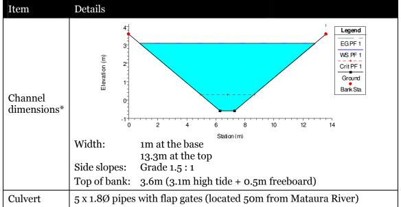
\*Channel dimensions are based on the flows from Waituna Lagoon only (5m<sup>3</sup>/s), and do not include the current channel flows.
