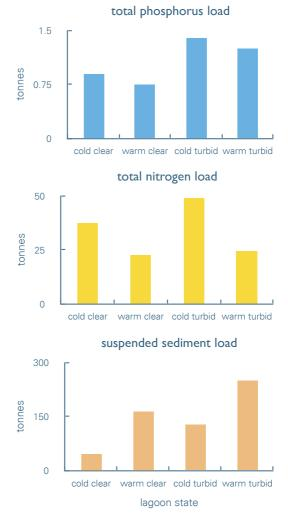
Figure A2-8. Estimated lagoon flushing loads of nutrients and suspended solids based on mean concentrations shown in Fig. A2-7.
