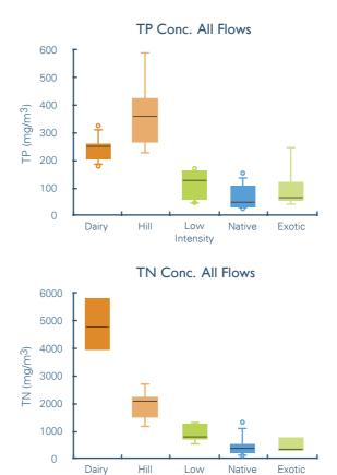
Fig. A1-6. Concentrations of total phosphorus (top) and total nitrogen (bottom) in streams draining catchments with different land uses. Values are temporally integrated, but not flow-weighted. The central solid line is the median value, the ends of the box are at the 25th and 75th percentiles, whiskers are at the 10th and 90th percentiles (where appropriate), and circles are outliers. Redrawn from Elliott & Sorrell (2002).
