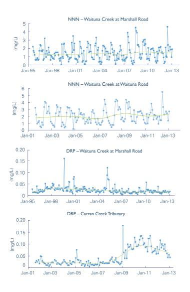
Fig A1-15. A weak upward trend in Nitrate-nitritenitrogen in Waituna Creek at Marshall Road. A Lowess smoothed line is fitted through the points.
