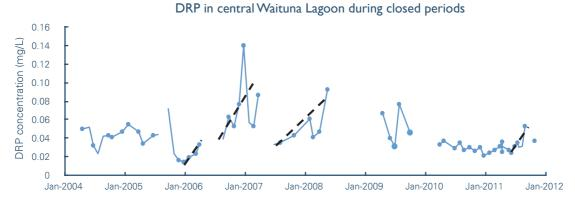
Fig. A1-11. Dissolved reactive phosphorus (DRP) concentrations in central Waituna Lagoon during closed periods. Dashed lines show where increasing DRP concentrations could suggest internal phosphorus loading to the lagoon. Data from Environment Southland.
