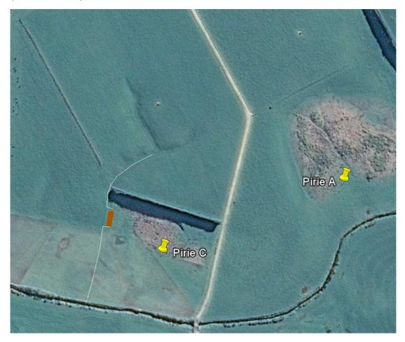
**Figure B-4: Potential site for wood-chip filter on Pirie Farm.** Subsurface drain flow to be diverted via weir into filter and then returned to drain at exit. High flow bypass via drain to be maintained.
