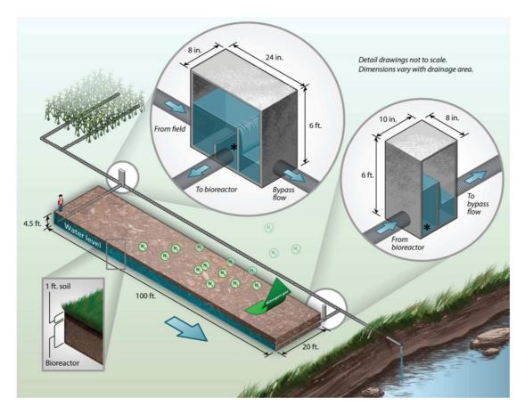
**Figure 6-1: Basic concept for wood-chip denitrification filters.** Diagram from (Christianson et al. 2012).
