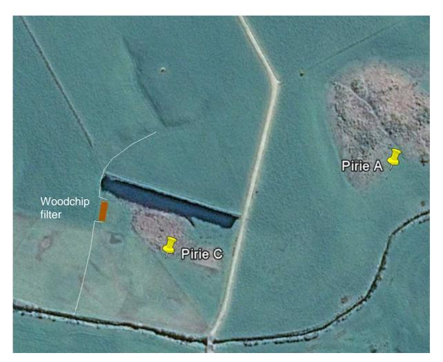
Figure 6-2: Proposed woodchip denitrification filter trial site Pirie C. Filter dimensions 5 m by 21 m x 1 m deep (105 m<sup>3</sup>) receiving subsurface drainage from a 9 ha catchment.
