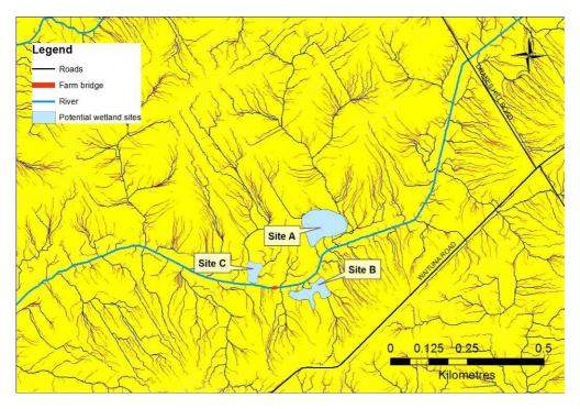
**Figure B-5: Pirie farm potential contributing catchments for site A-C.** The detailed drainage network (obtained from LiDAR data) illustrates the approximate areas that drain into the wetland sites.
