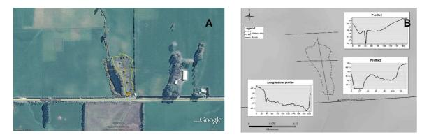
Figure A-16: Site 26 A. Satellite image of potential site. B. LiDAR contours and cross-sections.
