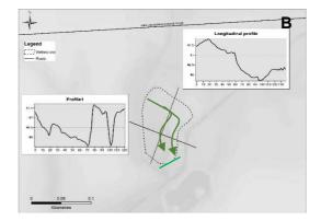
**Figure A-13: Site 4. A. Satellite photo of potential wetland site. B. LiDAR contours.** Potential bund site shown in green. Excavation of site would be required to induce flow distribution with sinuous path as shown in orange.
