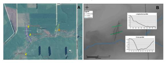
Figure B-2: A. Google Earth image of site 28 in August 2013. B. LiDAR contours and crosssections. Potential bunds shown in green and proposed wetland area shown by dashed line.
