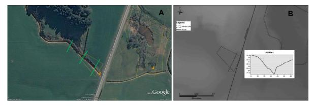
Figure A-19: Site 13b. A. Satellite image of potential CW site. B. LiDAR contours and crosssections. Note potential bund sites.
