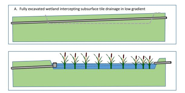
**Figure 4-1: Illustration of wetland creation in low gradient, tile-drained situations.** Note that to maintain the functioning of the upstream land areas the whole wetland needs to be excavated to below the upstream drain depth to maintain functioning of upstream drains.
