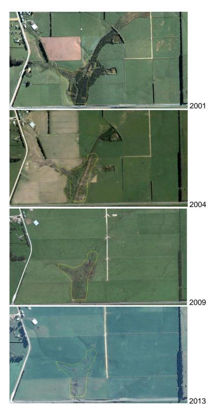
**Figure 3-2:** Location 2: Example of recent wetland drainage in the upper Waituna Catchment. Prospective sites for wetland construction investigated in the present study are marked. Various episodes of drainage works are visible in 2003 (not shown), 2004 and 2009 views.
