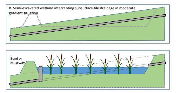
**Figure 4-2: Illustration of wetland creation in moderate gradient, tile-drained situations.** Note that in this case a bund can be used, reducing excavation requirements whilst maintain the drainage of upstream land.
