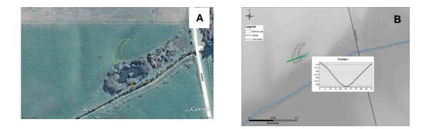
Figure A-8: A. Satellite photo of site. B. LiDAR contours. Potential bund shown in green. Bund may need to be >2.5m.
