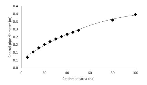
**Fig. 2**. Control pipe dimensioning for various catchment areas using a detention time of 2 days, a difference in the headwater and tailwater elevations of 0.3 m, a loss coefficient of 0.5, and a detention storage volume of 225 m<sup>3</sup>.
