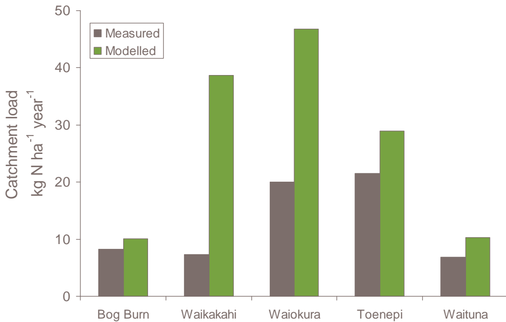
Figure 5 Measured and modelled losses of nitrogen in the streams draining the 5 intensively farmed catchments. Modelled losses of nitrogen from the farms were predicted by nutrient budget analyses.
