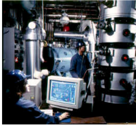
Experimental investigation of CO 2 -recycle combustion (courtesy of CANMET)
